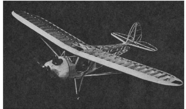
The construction is no more difficult than the ordinary gas buggy. Special designed nose will knock out in case of a hard landing, thus saving engine casualties.
