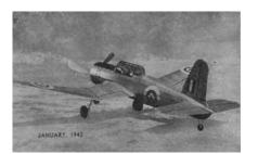
And it's realistic despite the emphasis on flying ability. Note the reversed gulled wings and the typical Vultee tail assembly. Colored circles are painted on.
